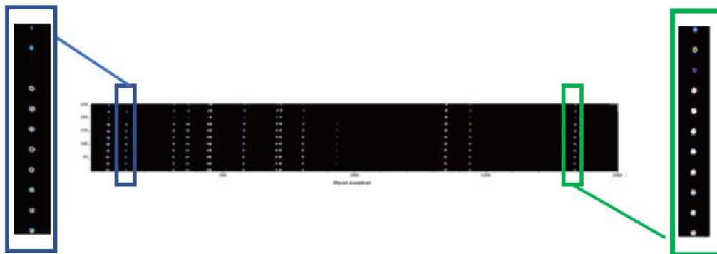
Fig. 4: Neon Spectrum in Imaging Mode 20-core fiber bundle / 100 \mu m core diameter
