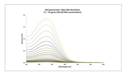
Even a small amount of protein contamination in DNA solution can have a large effect on UV absorbance. In this case, the SR4 demonstrated good linearity up to 2 AU.
